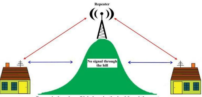
Communication only possible by bouncing the signal through the repeater
