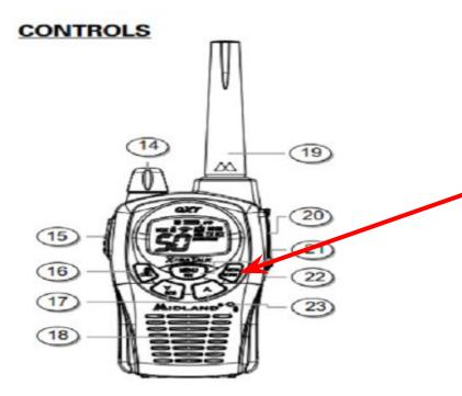
**SCAN** Your radio can scan all 50 channels for activity. To enter, quickly press the SCAN button. Repeat the same procedure to exit. Your radio will rapidly scan each of the 50 channels and stop on any active channel.
